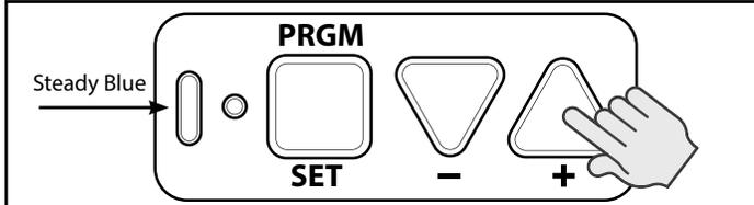
7. Release UP arrow button (+) and the round LED will begin flashing blue. (the long LED will go off.)
