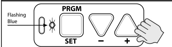
8. Press and hold the up arrow button (+) to begin opening the garage door. When the garage door is fully opened, release the up button (+). If it has gone too far press and release the down button (-) to move the door down slightly. The door can be moved up or down with the arrow buttons. Stop the carriage short of the opener powerhead. It is important for the red cord to be clear of the powerhead to allow for manual door operation.
