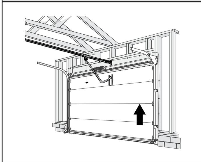
9. Press and release the program/set button—both LEDs flash blue and then go off.
