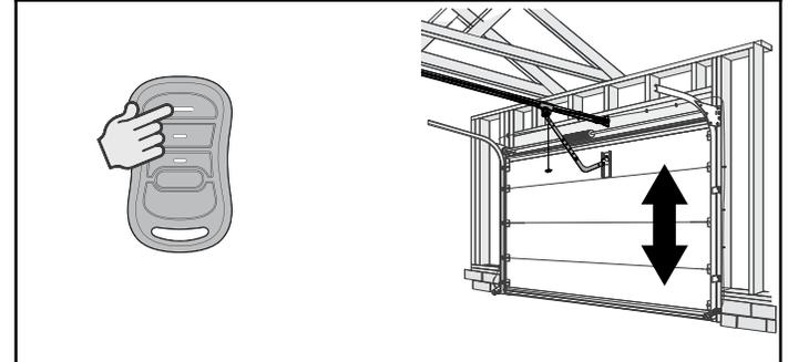
If the remote is successfully cleared, the round powerhead LED will flash blue when the remote button is pressed and the opener will not operate.
