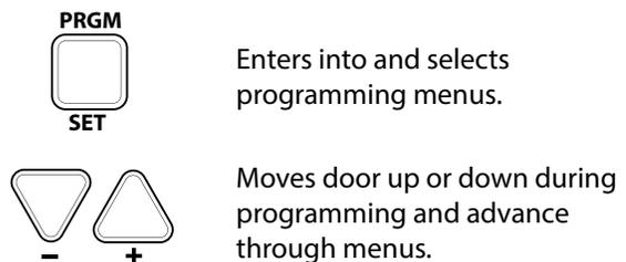
**NOTE:** While setting limits, the powerhead has a 30 second time-out period when none of the three programming buttons have been selected. If you see two solid red flashing LEDs or if the LEDs flash red three times and then go OFF, you have run out of time and must go back to the beginning of the travel limit setting step.
