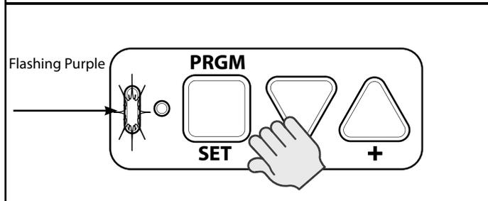
3. Press and hold the UP (+) and DOWN (-) button at the same time, until both LEDs flash blue and go off.
