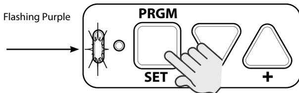
B. Press the chosen HomeLink button for two seconds and release. Press that same button again for two seconds and release. The long LED will flash blue and then turn off.
