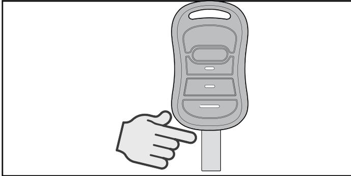
2. Press and hold the program button on the opener for two seconds until the round LED turns blue, then release. The long purple LED will flash.
