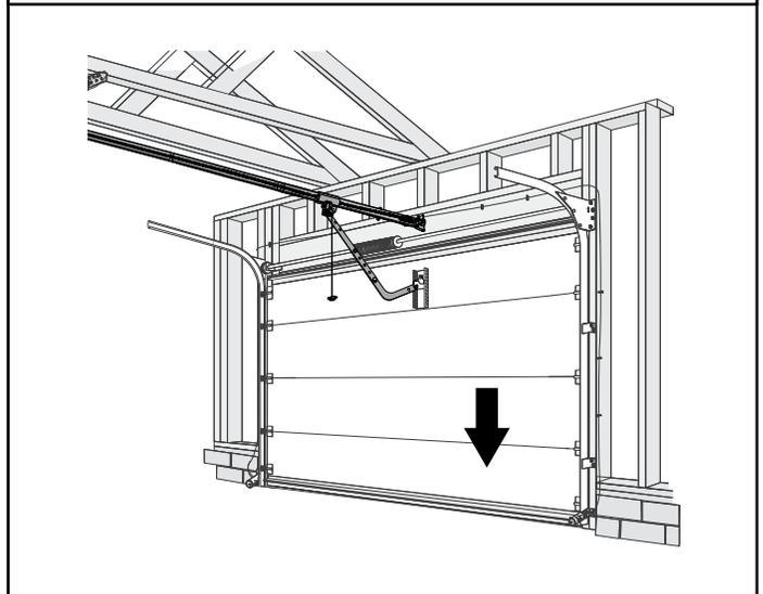
5. Press and release the program/set button—both LEDs flash blue and then go off. **The DOWN (CLOSED) TRAVEL LIMIT IS NOW PROGRAMMED.**
