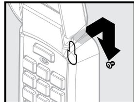
5. Mark and drill a pilot hole for the bottom screw (included) and secure keypad to wall (**DO NOT** overtighten).
