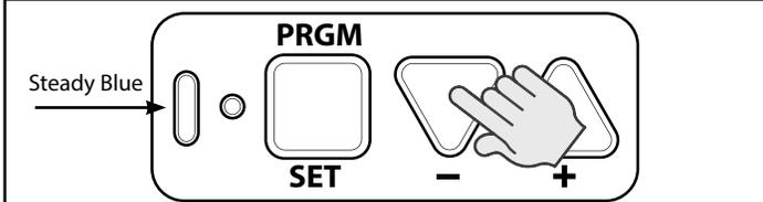
3. Release down arrow button (-) and the long LED will begin flashing blue. (Round LED still off.)
