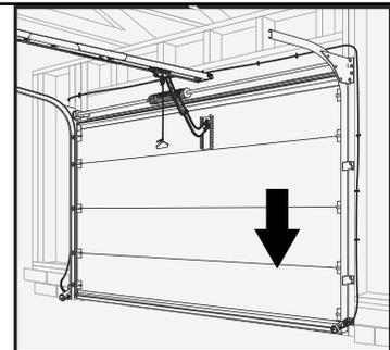
When the door contacts the board, it should stop and reverse direction within 2 seconds to the fully open position. Long LED light on the powerhead will begin to flash RED with the reversal of the door. Remove the 2" x 4" board after a successful contact reversal test. The next cycle will clear the flashing red LEDs.
